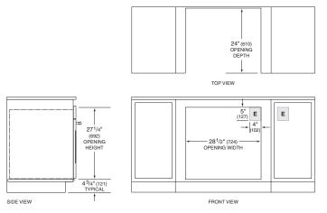
NOTE: Location of electrical supply within opening may require additional cabinet depth. Dashed line represents profile of unit.
