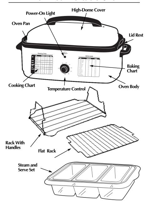
**High-Dome Cover** is designed to control heat and moisture efficiently. **Important:** When removing the cover from the oven during or after cooking, lift the cover away to avoid contact with escaping steam.
