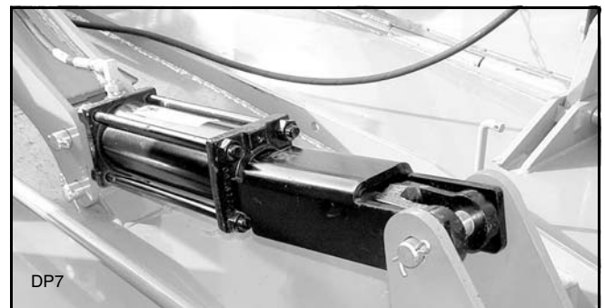
Figure 3. Transport Lock In Transport Position
