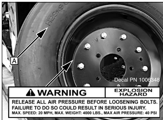
Figure 26. Split Rim Tire Servicing
