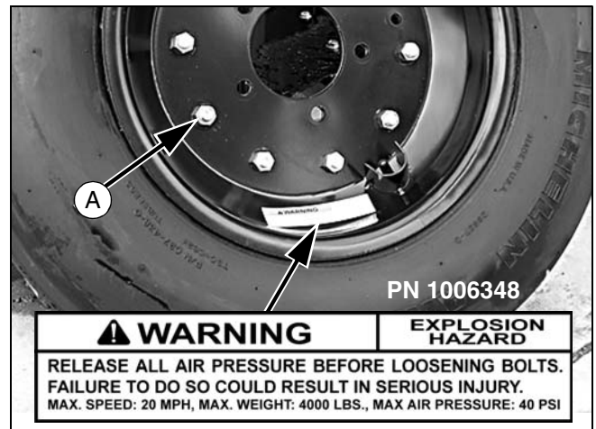
Figure 9. Split Rim Tire Servicing
