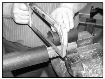
Figure 4. Cut Shaft to Length
