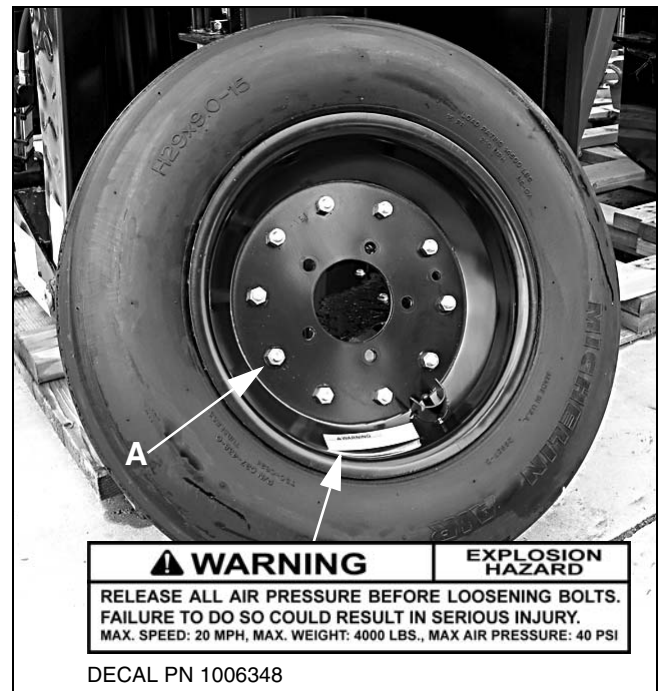
Figure 17. Split Rim Tire Servicing
