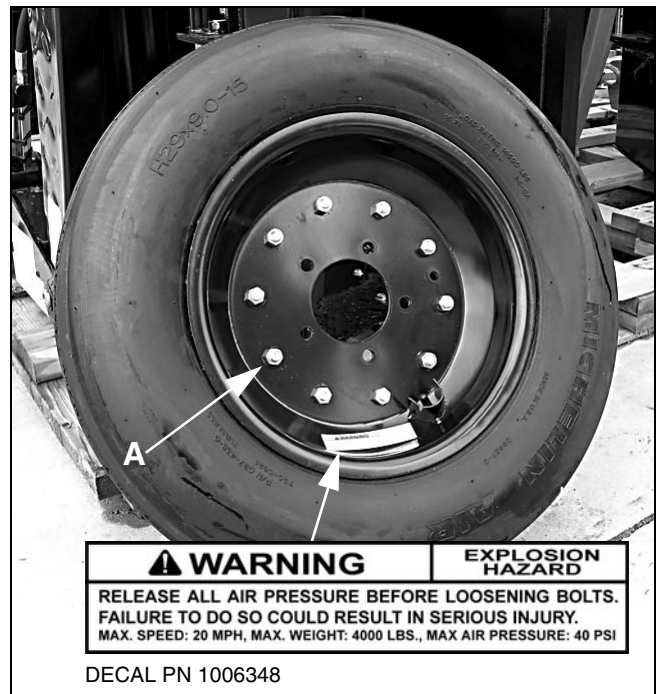
Figure 32. Split Rim Tire Servicing
