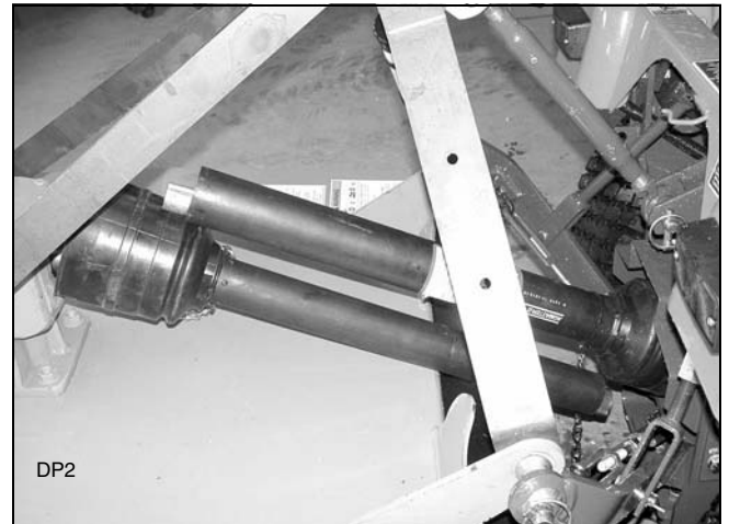
Figure 6. Drive Halves Placed Parallel
