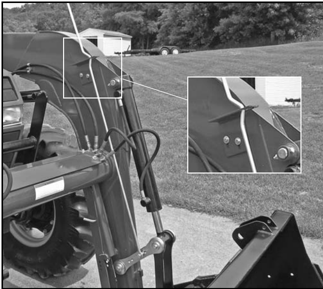
Figure 40. Bucket Level Indicator Installed
