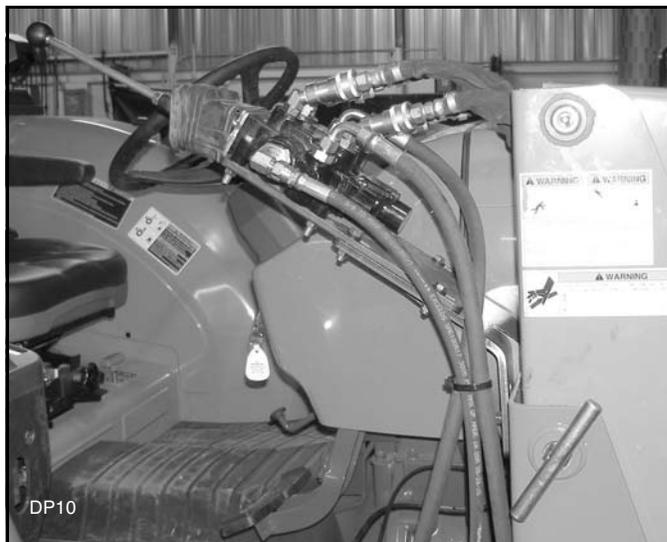
Figure 43. Control Valve Installed (Typical)
