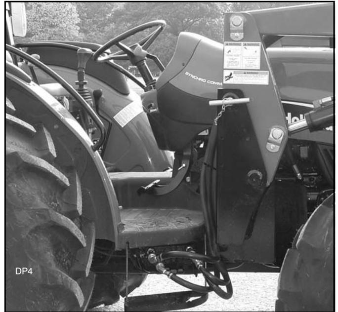
Figure 31. Tractor Remote Control Lever
