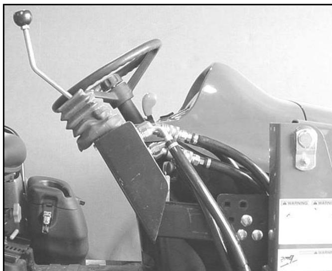
Figure 13. Control Valve Installed
