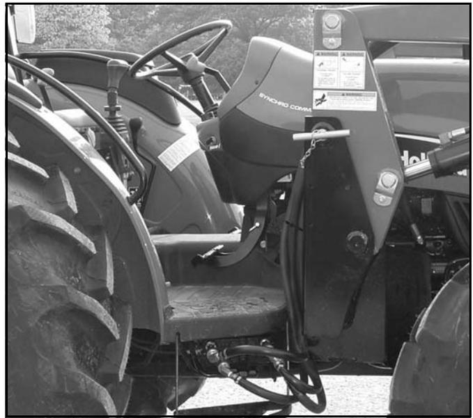
Figure 24. Tractor Hydraulic Control Lever and Valve
