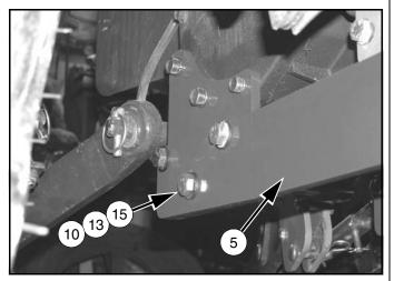
Figure 4. Right Rear Rail to Axle Plate Connection
