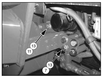
Figure 1. Right Rear Mount Installed
