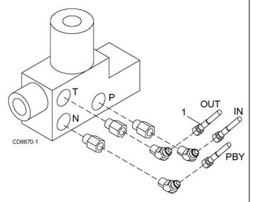
Figure 19. Hydraulic Hose Installation Hydraulic Manifold
