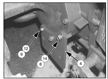
Figure 3. Axle Plate Installed, Left Side Shown
