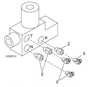
Figure 17. Hydraulic Fitting Installation
