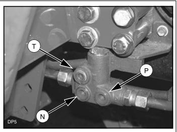
Figure 15. Tractor Hydraulic Manifold
