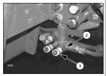
Figure 16. Hydraulic Fittings Installed
