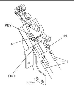
Figure 18. Hydraulic Hose Installation - Control Valve
