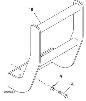
Figure 6. Grill Guard Installation
