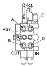
A - BUCKET CYL. BASE END (DUMP) - RED B - BUCKET CYL. ROD END (ROLLBACK) - BLUE C - BOOM CYL. ROD END (DOWN) - YELLOW D - BOOM CYL. BASE END (UP) - GREEN
