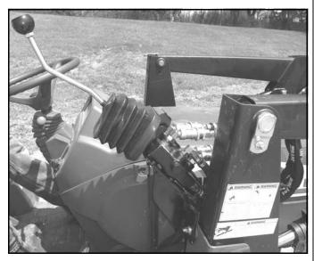
Figure 14. Single-Lever Control Valve
