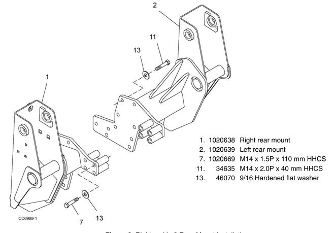
Figure 2. Right and Left Rear Mount Installation
