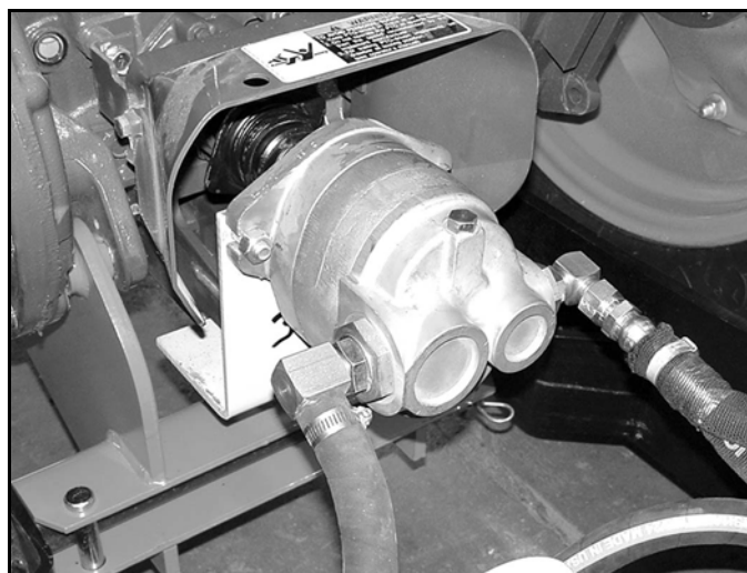
Figure 15 Pump & Bracket Installed
