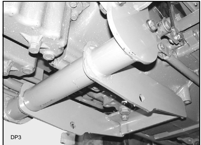
Figure 3 Crossmember Installed with LMK #111768
