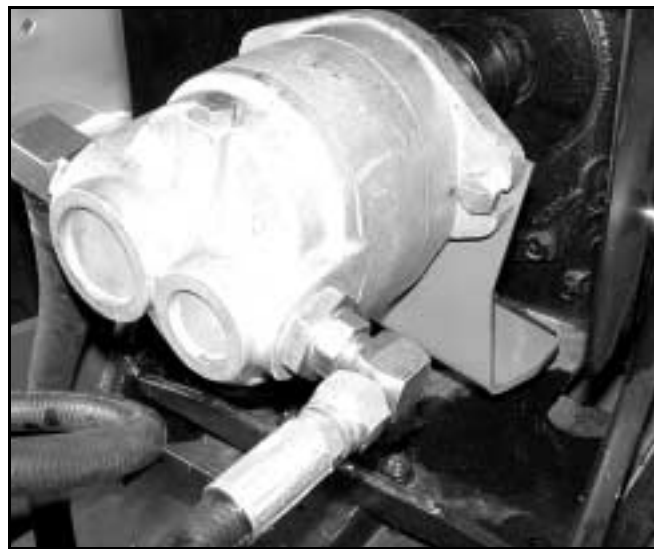
Figure 12 Pump and Bracket Installed
