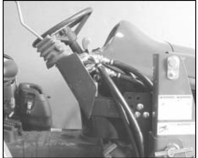
Figure 12 2-Spool Control Valve Installed (Typical installation)
