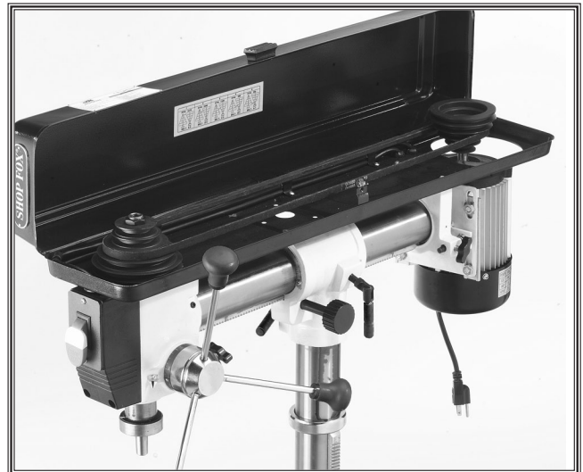
Figure 36. Adjusting belt to desired speed.
