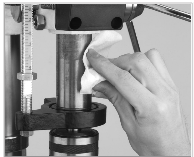
Figure 25. Clean and oil quill shaft.
