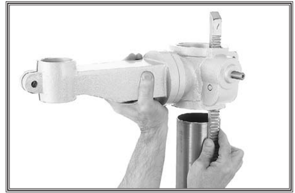
Figure 11. Sliding table bracket and rack over column.
