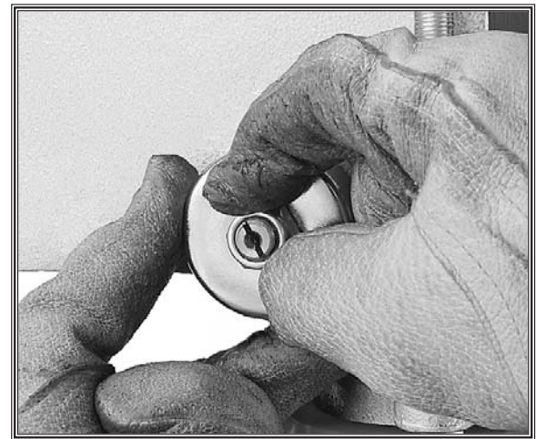
Figure 32. Loosening spring nut.
