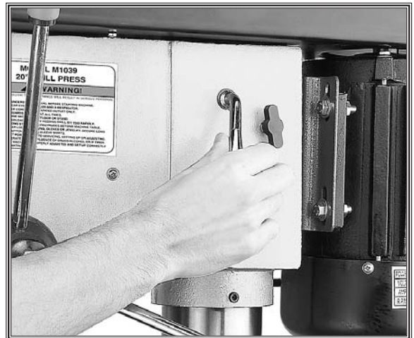
Figure 24. Using the belt tension lever.
