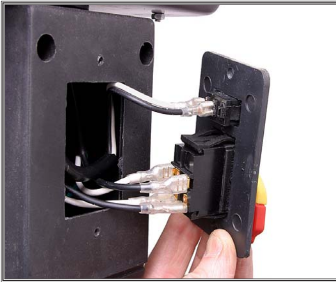
Figure 33. Power and light switch wiring.
