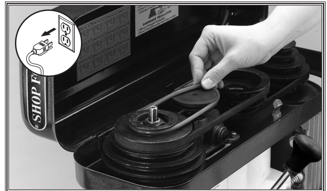
Figure 44. Stretch the belt to fit on pulleys.
