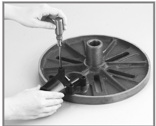
Figure 9. Installing the dust port.
