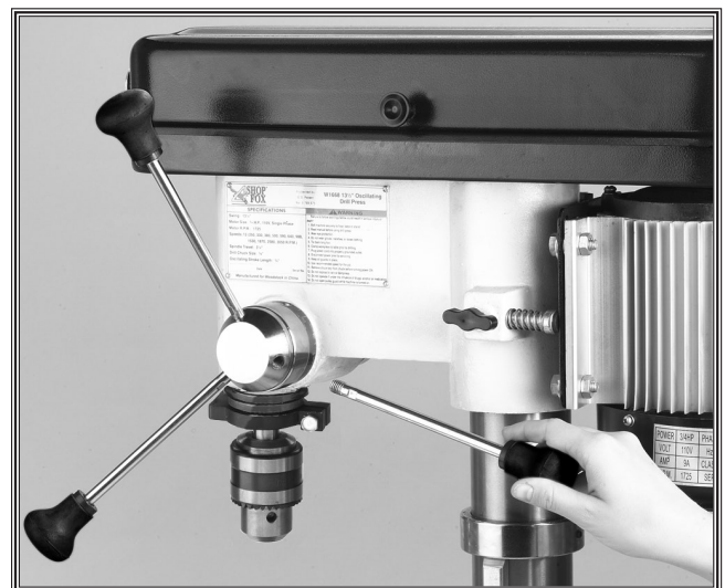
Figure 21. Installing spindle handles.
