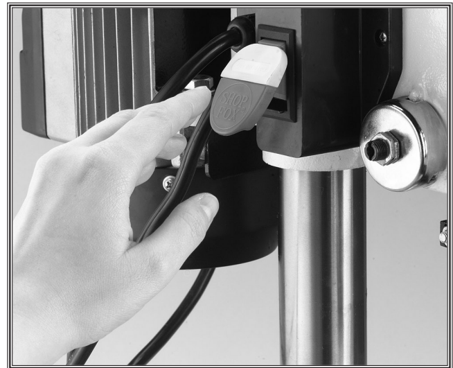
Figure 39. Hand poised over a typical stop switch.
