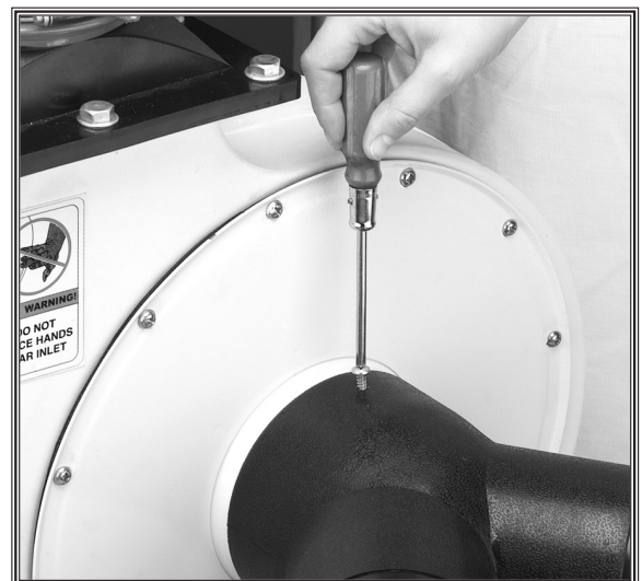
Figure 20. Securing inlet with screw.
