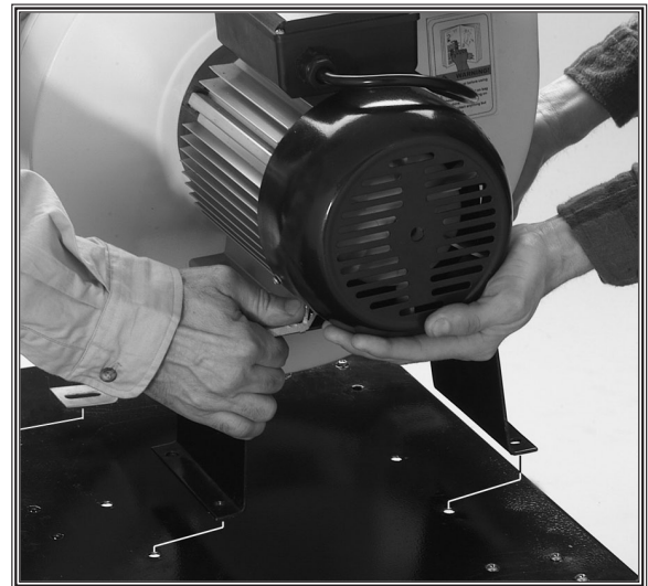
Figure 10. Motor/impeller assembly positioning.
