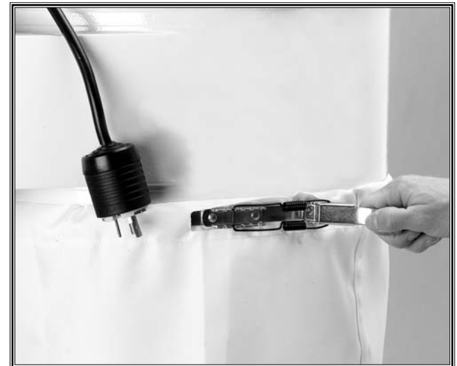
Figure 4. Unplug machine when changing bags.
