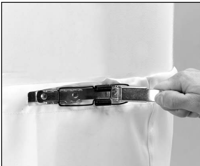
Figure 15. Securing the lower bag quick-release band clamp.
