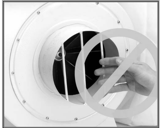
Figure 2. Keep hands away from impeller.
