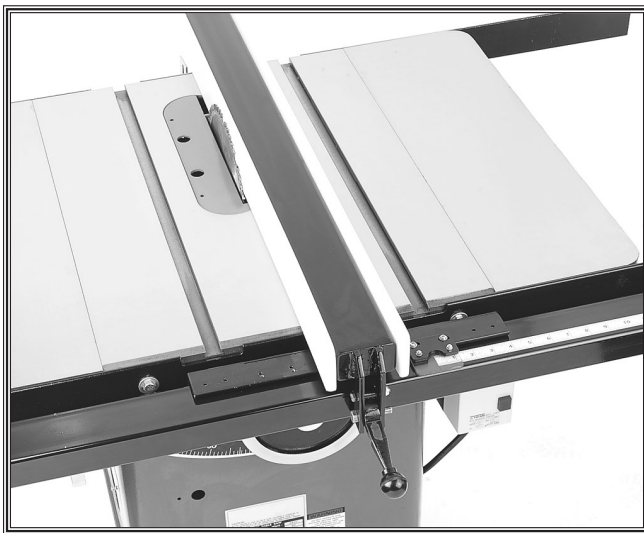
Figure 12. Fence contacting the blade.
