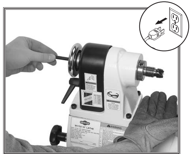
Figure 11. Removing spur center using knock out bar.
