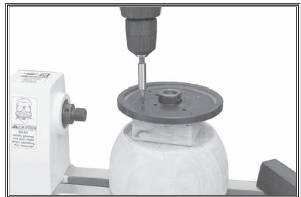
Figure 24. Typical example of mounting faceplate to a backing block.
