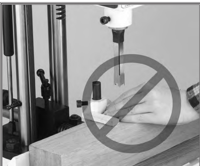
Figure 6. Never place hands under chisel.
