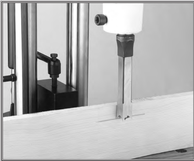
Figure 32. Use penciled line to gauge depth.
