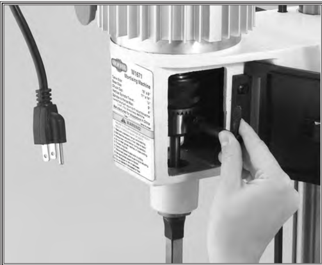
Figure 2. Unplug before changing chisels.
