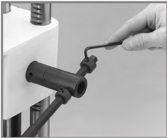
Figure 11A. Secure collar onto hand lever.
