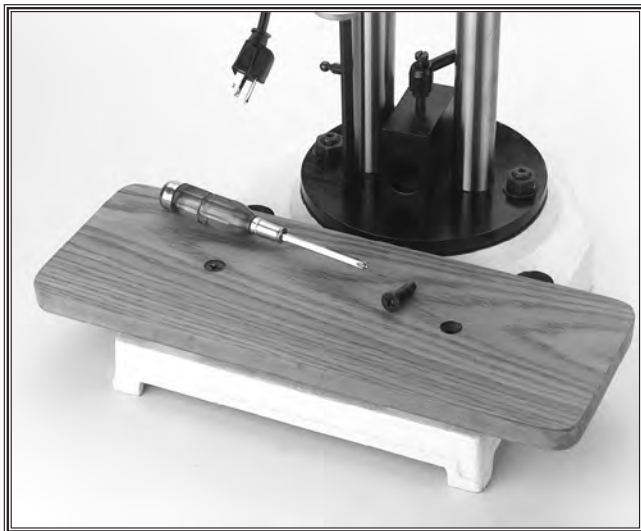
Figure 14. Work table secured with screws.
