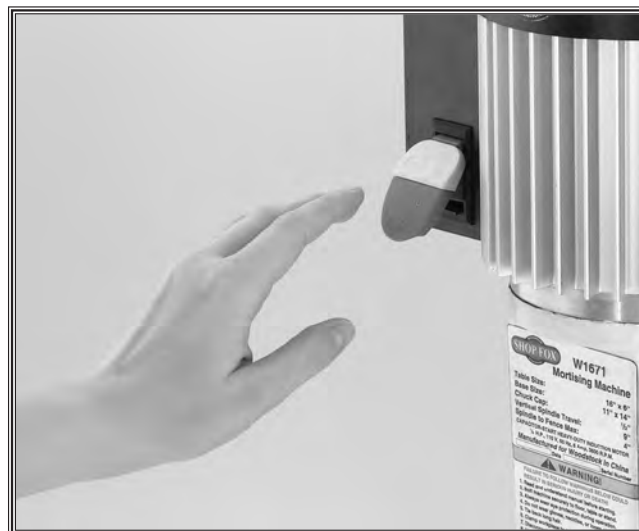
Figure 30. Hand poised over stop paddle.
