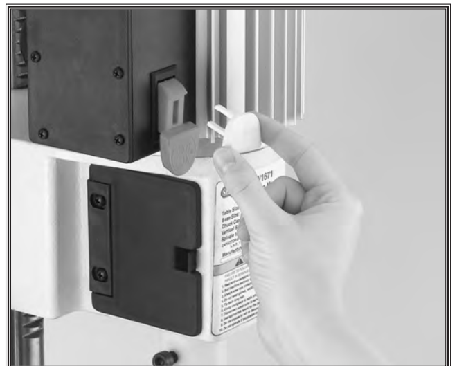
Figure 5. Remove safety key when not in use.
