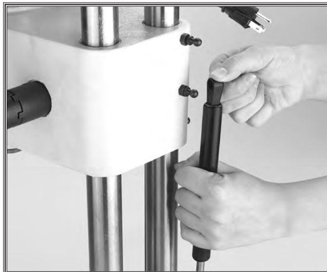
Figure 13. Compressing gas spring to assemble.
