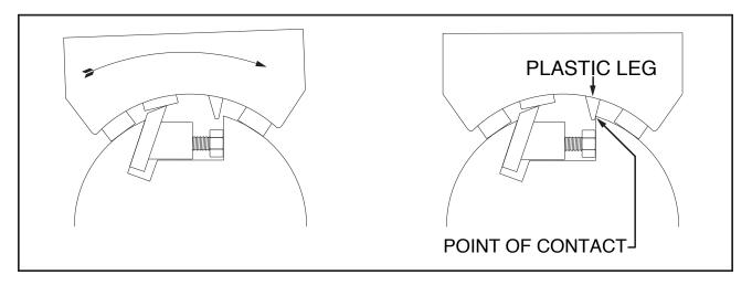
6. Hold the cutterhead with one hand and slide each jig until the indexing pin contacts the back edge of the gib slot. See Figure.
