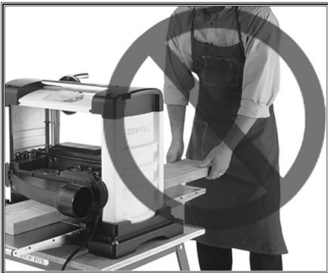
Figure 3. DO NOT stand directly behind workpiece line of travel.
