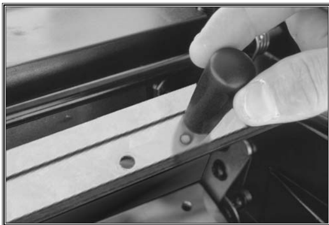
Figure 19. Lift out the locking plate with the magnets.
