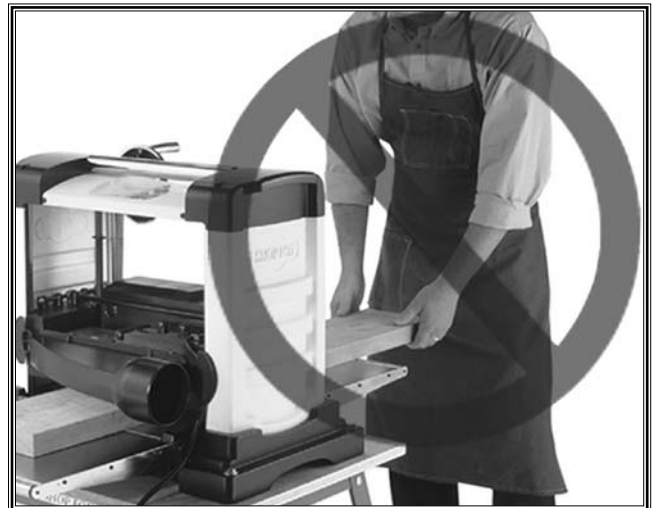
Figure 32. DO NOT stand in the path of the planer outfeed because you can be hit with the workpiece.
