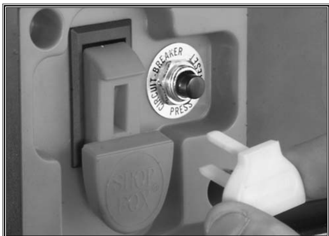
Figure 28. Remove the safety lockout key.
