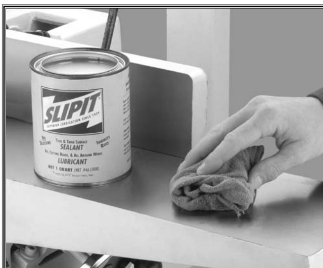
Figure 43. Applying lubricant to table surface.
