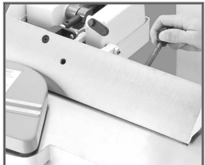
Figure 32. This is the fence in the 45° R position.
