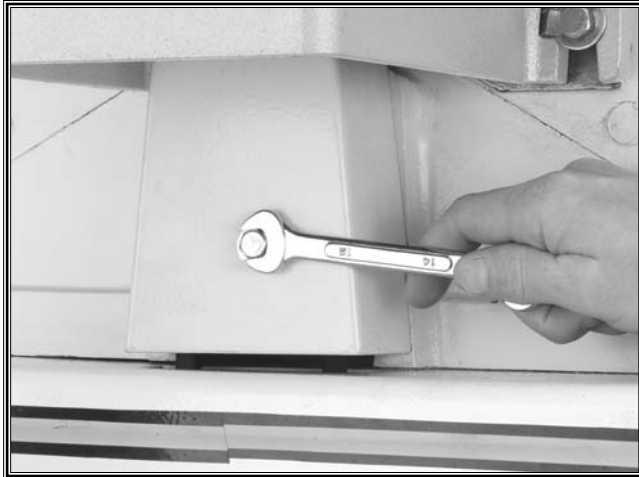
Figure 18. Attach belt guard to stand with the hex bolt.
