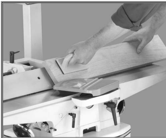
Figure 40. This is an example of a bevel cutting operation with the fence set at 45°.
