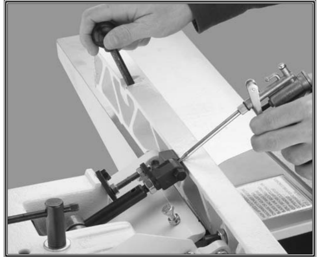
Figure 44. Lubricating fence pivot points.
