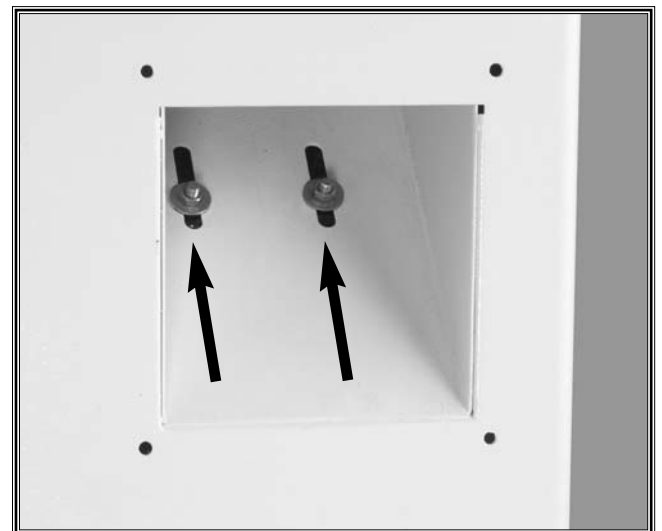
Figure 11. Motor mount bolts inside dust chute (two are not shown).
