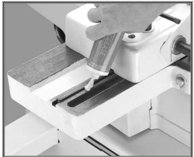
Figure 45. Greasing fence keyway.
