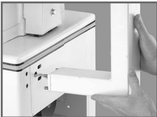
Figure 20. Mounting pedestal switch to stand.
