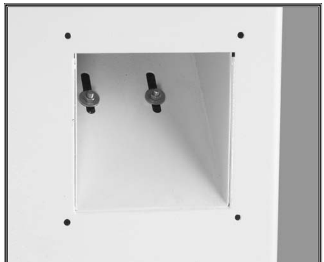
Figure 46. Motor mount bolts located in dust chute.
