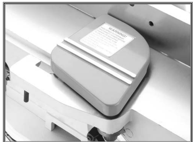
Figure 17. Guard in proper position against the fence and completely over the cutterhead.
