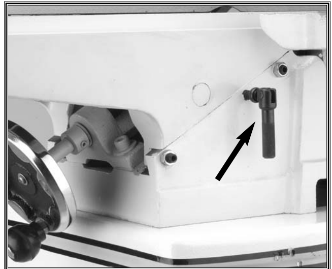
Figure 25. This is the outfeed table lock handle.
