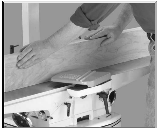
Figure 38. This is an example of an edge jointing operation.
