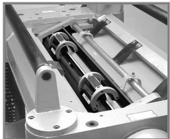
Figure 20. Planer Pal jigs holding knives for superior adjustment.
