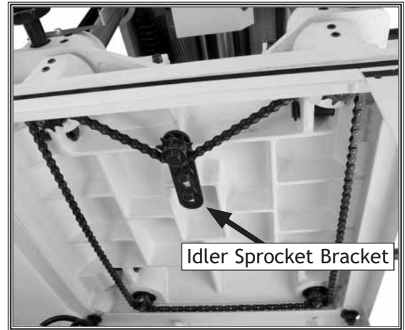
Figure 34. Chain drive system.
