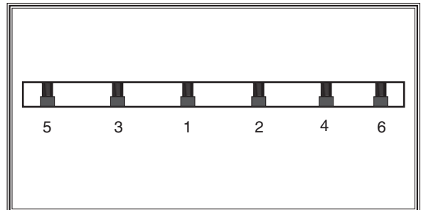
Figure 23. Gib bolt tightening sequence.
