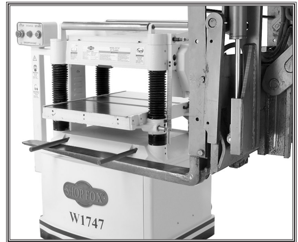
Figure 4. Example of planer being lifted using forklift.
