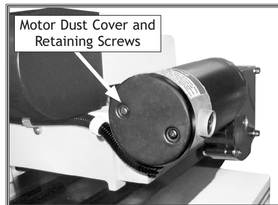
Figure 52. Feed motor end view.
