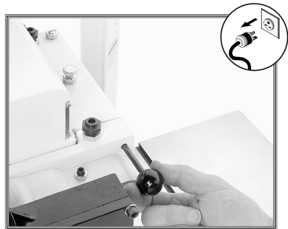
Figure 17. Removing the chip deflector.
