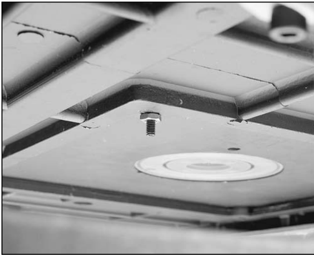
Figure 14. Leveling setscrew and jam nut.
