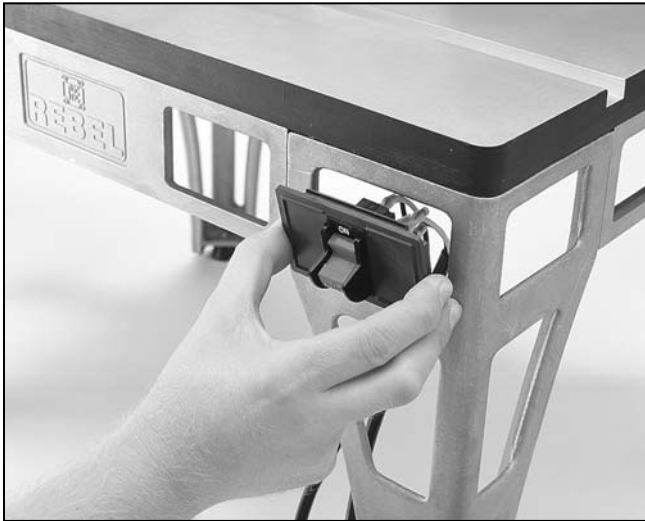
Figure 9. Installing the switch.
