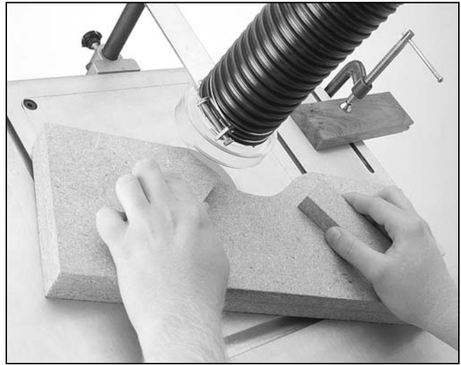
Figure 27. Work is supported by the guide bearing.
