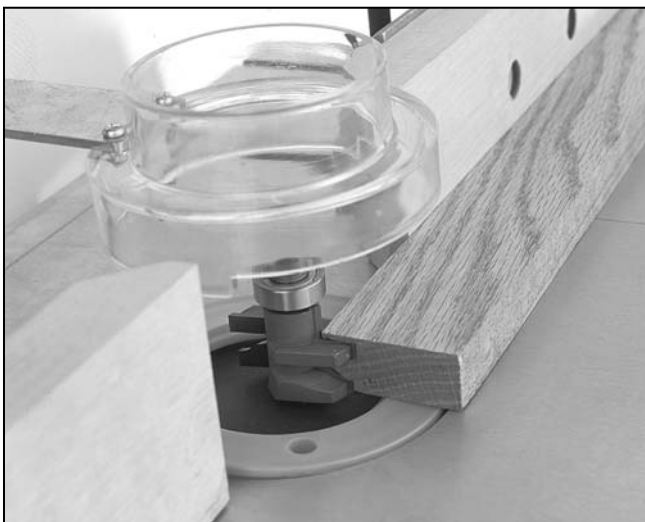
Figure 16. Gauge position of infeed fence with a sample piece of wood.
