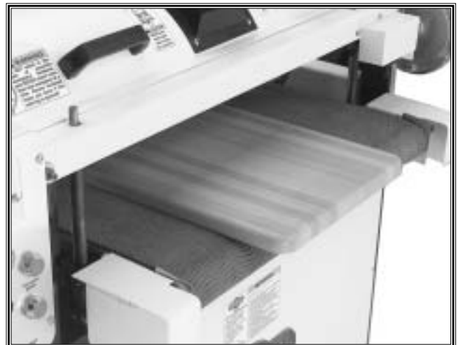
Figure 6. ALWAYS feed the sander with only one piece of stock at a time.
