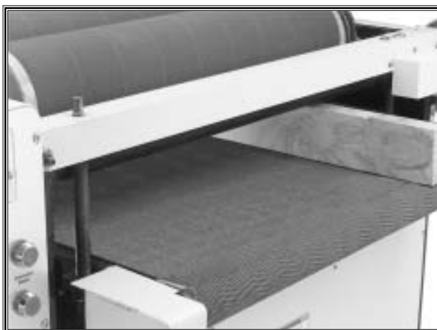
Figure 32. The 30" gauge block positioning.
