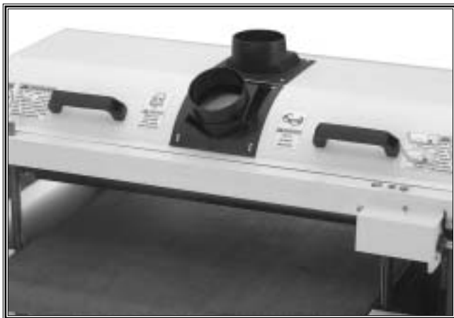
Figure 12. Dust ports and handles installed.
