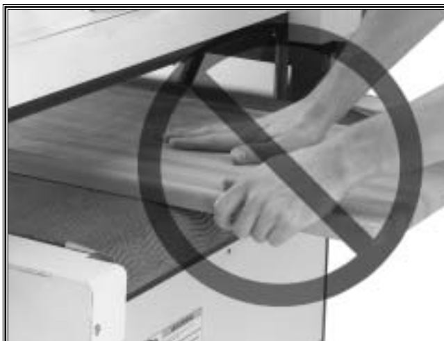
Figure 48. NEVER hold the workpiece where the conveyor and workpiece can pinch your fingers.
