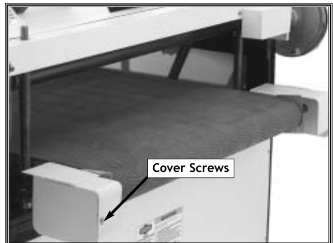
Figure 40. Infeed-conveyor safety covers.
