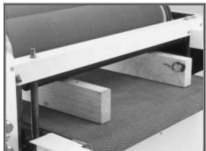
Figure 35. Two gauge blocks in position.
