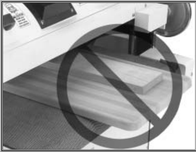
Figure 7. NEVER sand stock using a “sled” (another board) under the workpiece.
