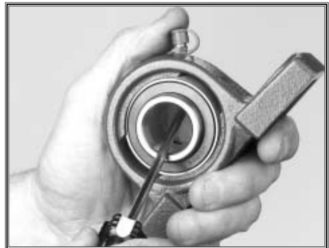
Figure 58. Bearing positioning for removal.
