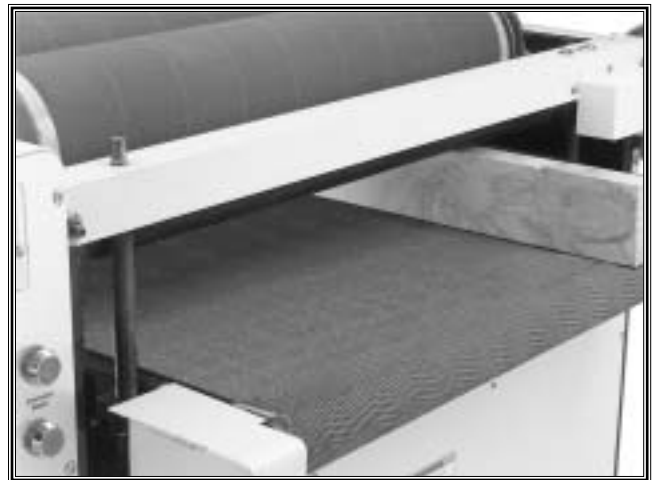
Figure 28. The 30" gauge block positioning.
