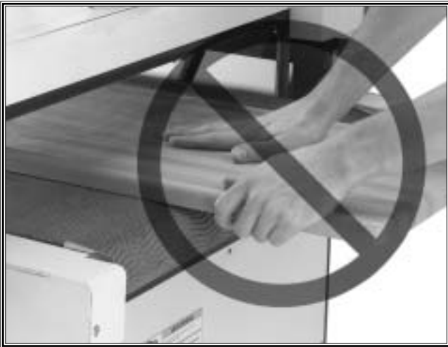
Figure 1. NEVER hold the stock where the conveyor and stock can pinch your fingers.
