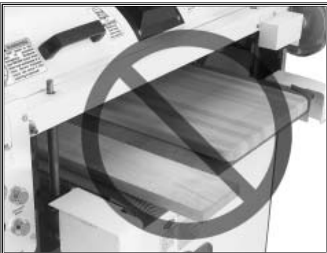
Figure 5. NEVER sand more than one piece of stock at a time.
