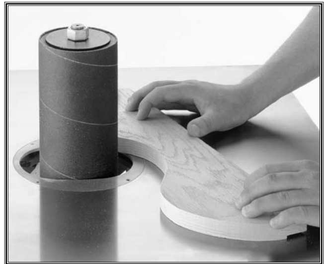
Figure 18. The Model W1686 is best suited for smoothing the curved cuts made by a bandsaw or jigsaw.
