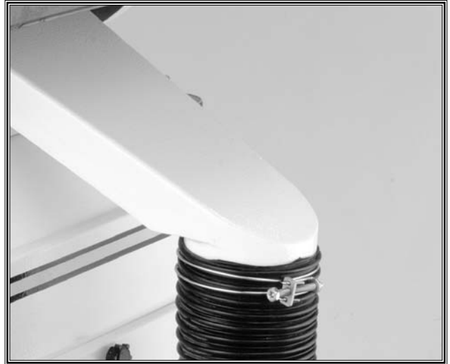
Figure 5. Attach a dust collection system to the 4" dust port to reduce the amount of uncontained dust.
