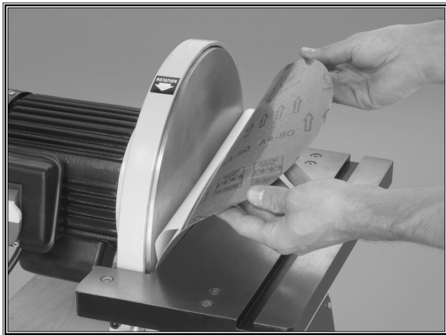
Figure 8. Slide covered sandpaper between disc and table.
