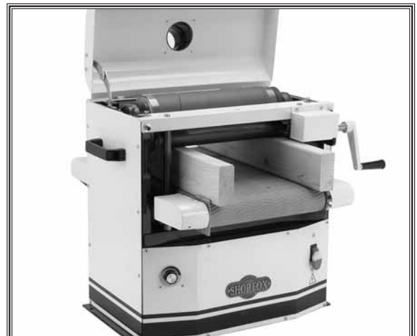
Figure 27. Gauge boards in position.
