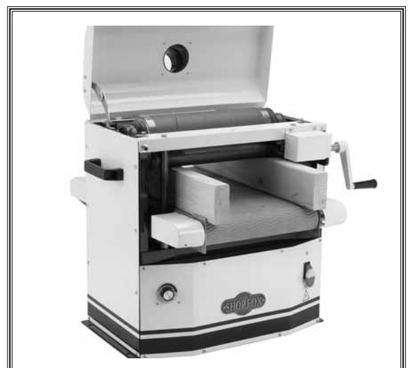
Figure 27. Gauge boards in position.
