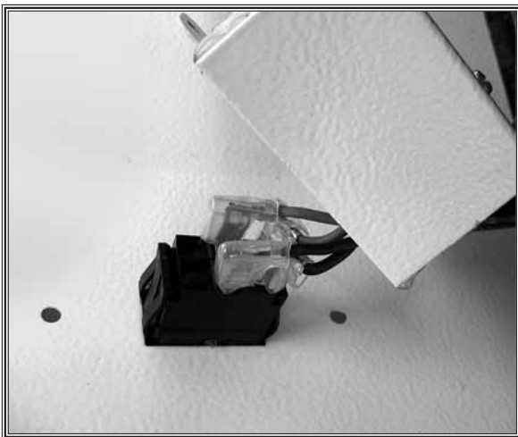
Figure 61. Main power switch.
