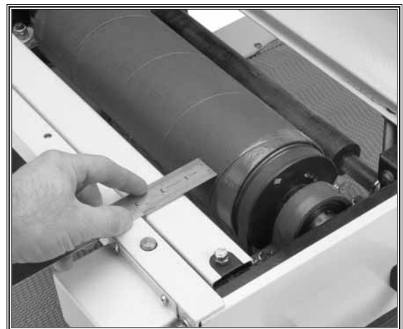
Figure 33. Measuring drum alignment.
