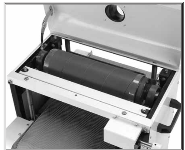
Figure 13. Sandpaper installed and taped.
