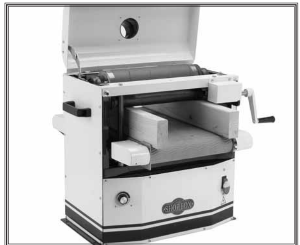
Figure 30. Gauge boards in position.
