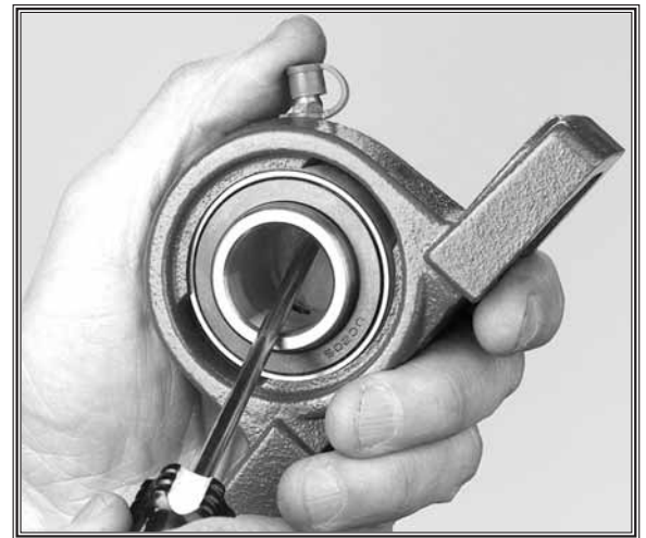
Figure 56. Bearing positioning for removal.
