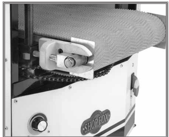
Figure 49. Conveyor belt loosened at the front adjustment bolts.
