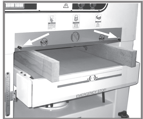
Figure 10. Pressure roller height adjustment locations and gauge boards installed.
