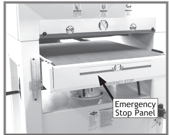
Figure 16. Emergency stop panel.
