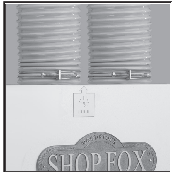
Figure 7. Dust collection hoses attached to dust ports.
