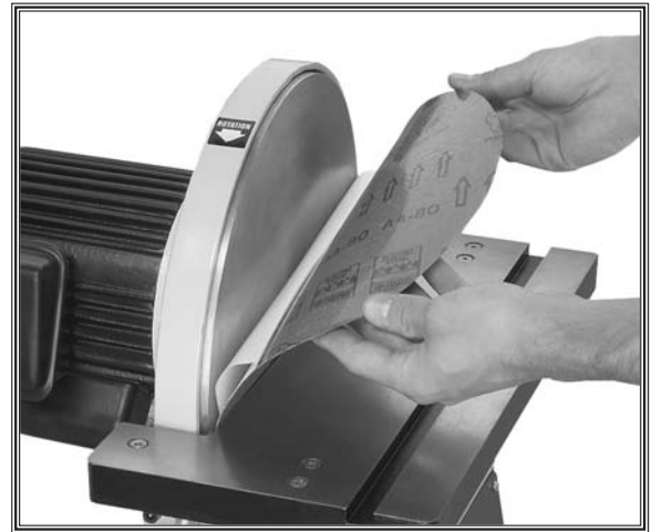
Figure 14. Slipping covered sandpaper between disc and table.
