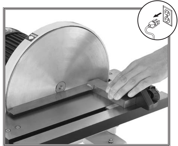
Figure 20. Squaring miter gauge to disc.
