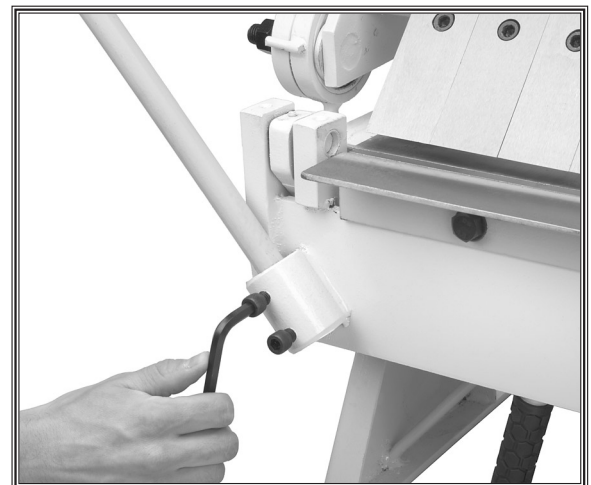
Figure 7. Mounting the counterweight.
