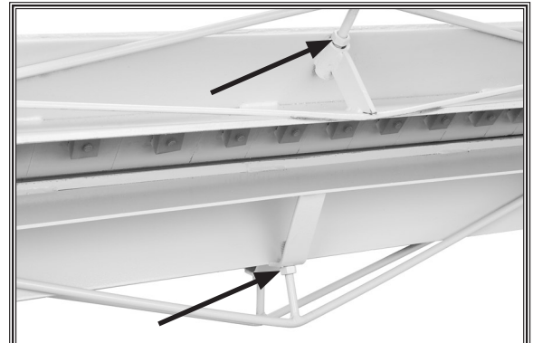
Figure 18. Bending wing mounting bolts.
