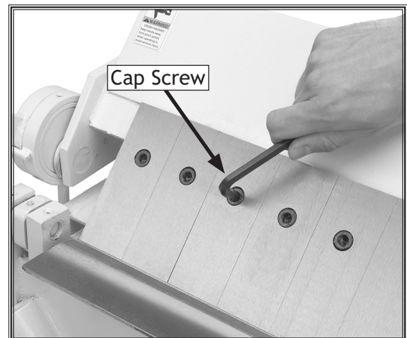
Figure 12. Top cap screw for loosening finger in order to slide it off the front guide.
