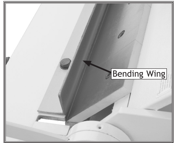
Figure 8. Bending wing moved approximately perpendicular to fingers to act as a straightedge.
