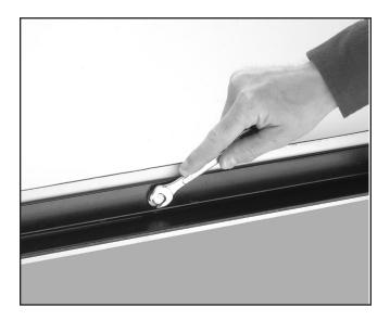
**Step 12.** Use the straightedge to verify that the extension table is flush with the saw table and is even along its entire length. Minor adjustments may be made by adjusting the rail-to-table hex bolts or by rotating the feet. *Note—lock the <sup>1</sup>/<sub>2</sub>"-12 hex nuts to keep the feet in place after adjustments are final.*
