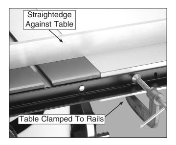
**Step 11.** Attach the rails to the table with the (8) <sup>3</sup>/<sub>8</sub>"-16 x 1<sup>3</sup>/<sub>4</sub>" hex bolts, (16) <sup>3</sup>/<sub>8</sub>" washers and (8) <sup>3</sup>/<sub>8</sub>"-16 nuts. The assembly order should be hex bolt, flat washer, rail, extension table, flat washer, and hex nut. *Note—some assemblies will require* <sup>3</sup>/<sub>8</sub>" *holes drilled through the table to match fence rail holes for mounting.*
