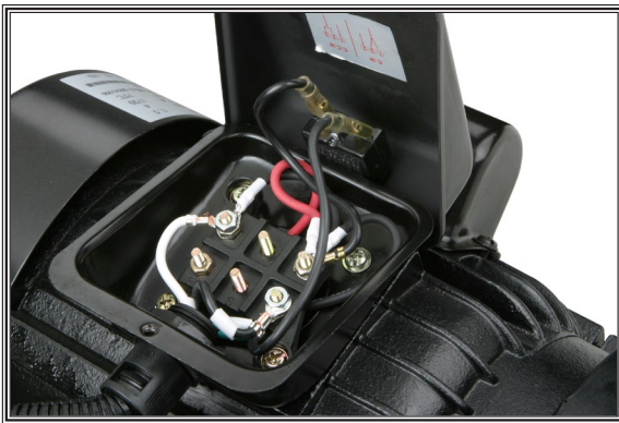
Figure 42. Junction box (M1).
