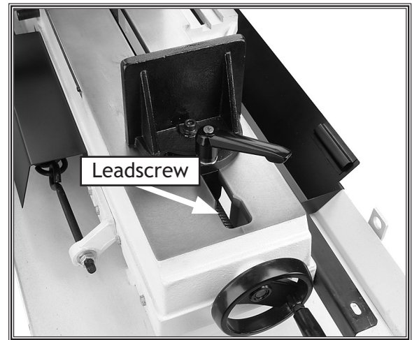
Figure 28. Vise leadscrew lubrication area.
