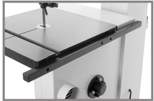
Figure 13. Rear fence rail attached to table.
