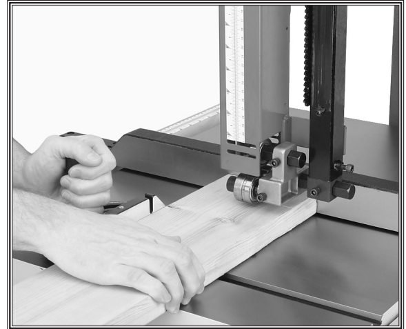
Figure 41. Typical crosscutting operation.
