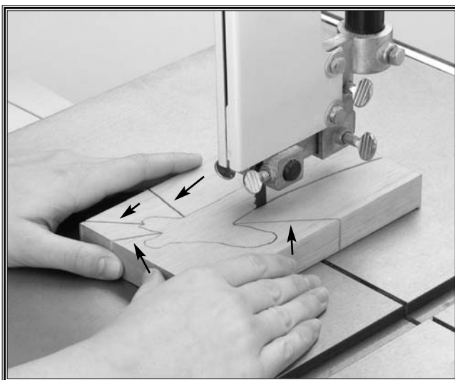
Figure 52. Relief cuts before cutting curves.
