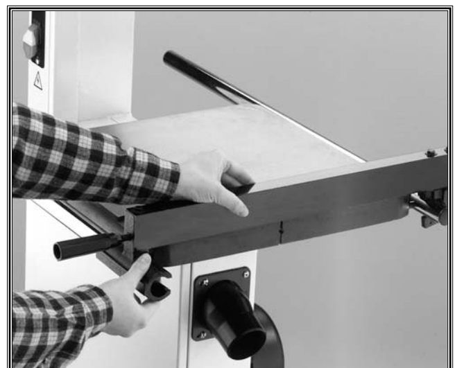
Figure 23. Starting fence on rail.
