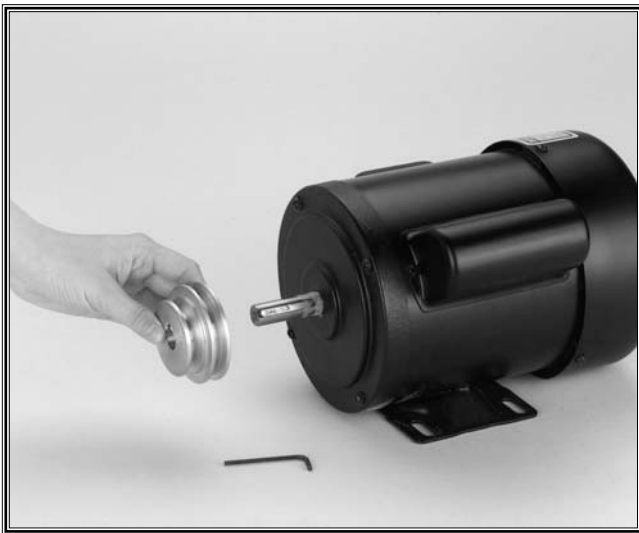
Figure 14. Installing pulley on motor.
