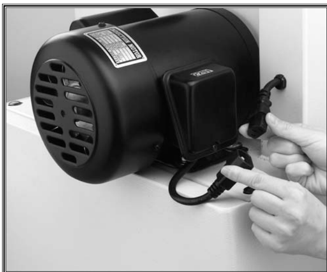
Figure 16. Plugging motor to switch.
