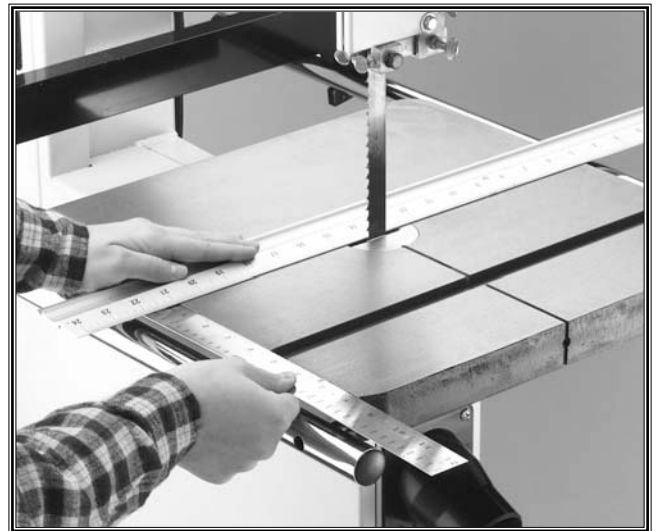
Figure 45. Squaring miter slot to blade.
