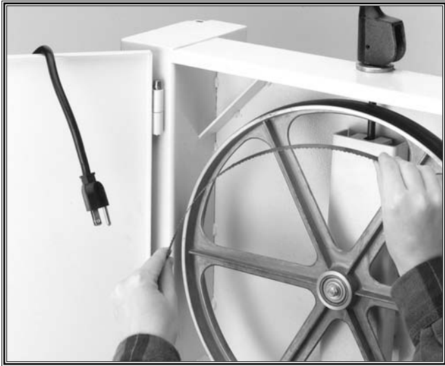
Figure 3. Unplug saw before changing blades.
