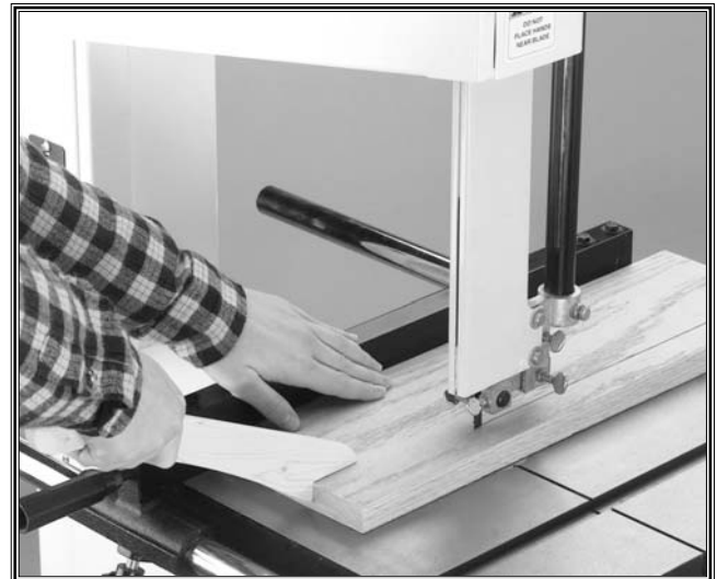
Figure 49. Ripping a board.
