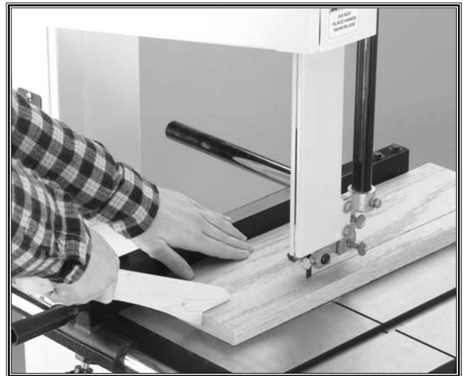
Figure 6. Use push sticks whenever possible.
