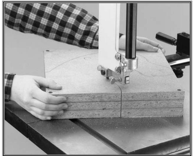
Figure 54. Making a stacked cut.
