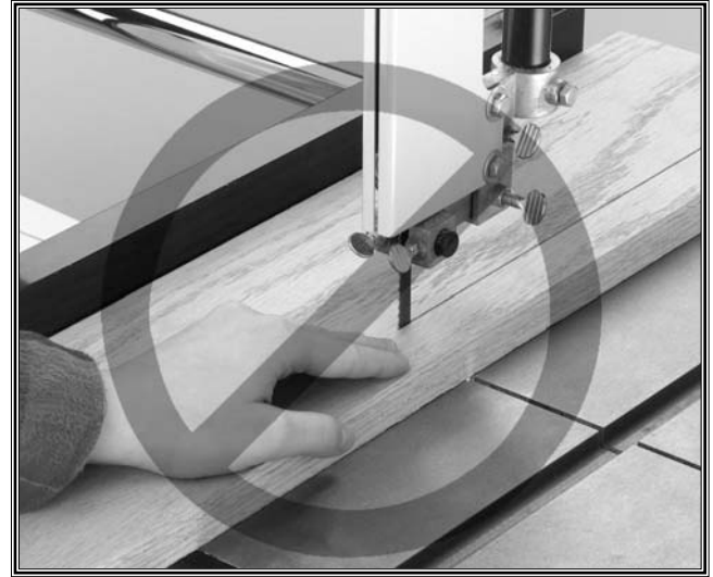
Figure 8. Never place hands in line of cut.
