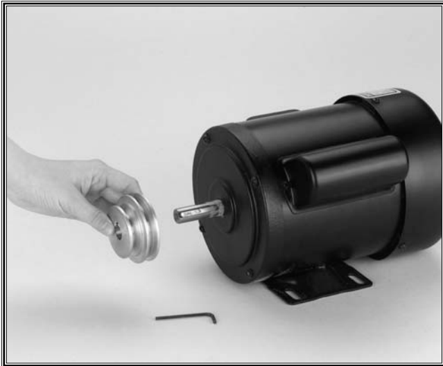
Figure 14. Installing pulley on motor.
