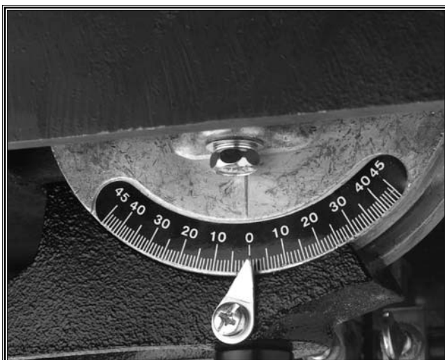
Figure 43. Pointer set to zero.
