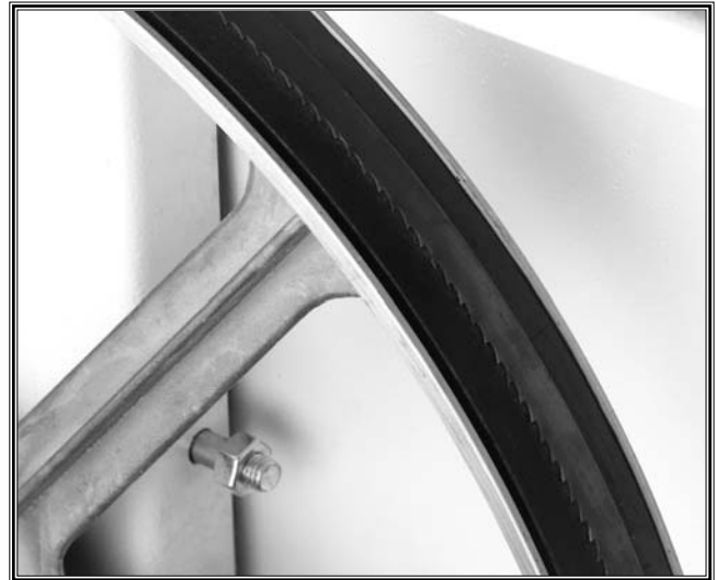
Figure 32. Blade centered on wheel.
