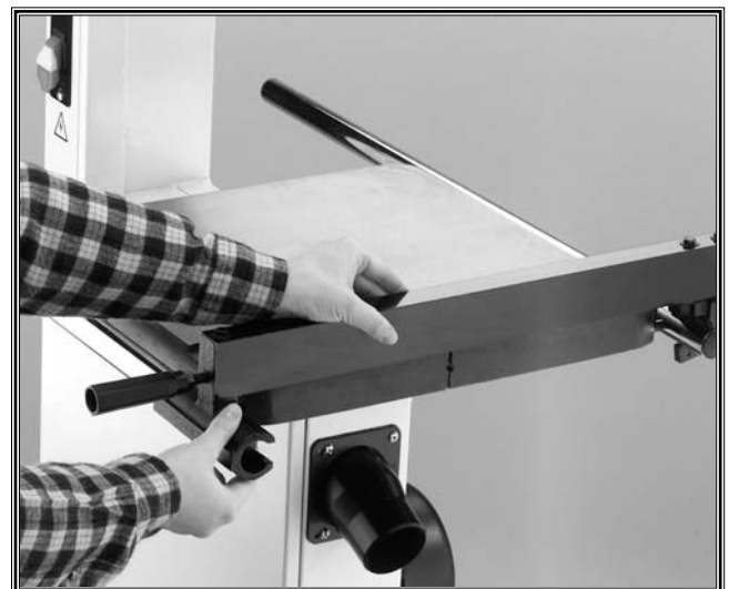
Figure 23. Starting fence on rail.
