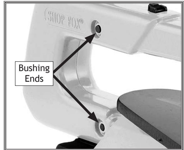
Figure 16. Plastic caps removed to expose the arm bushing ends.
