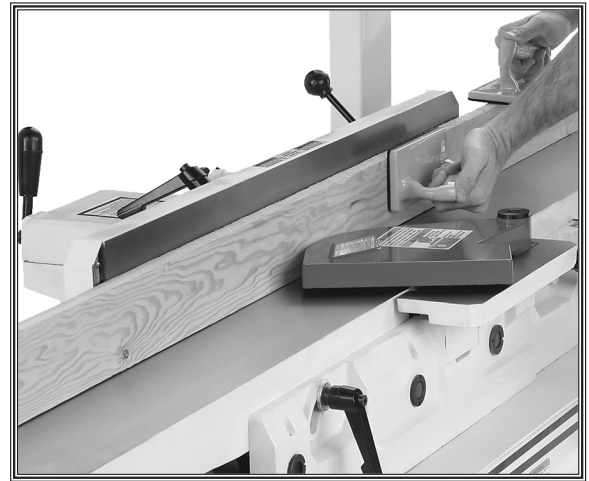
Figure 38. Typical edge jointing operation.
