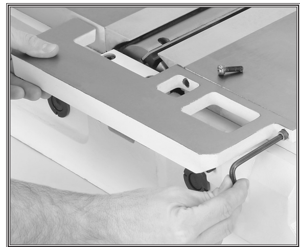
Figure 16. Attaching extension table to jointer.
