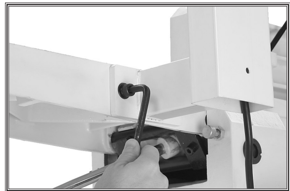
Figure 23. Attaching pedestal switch to the back of the jointer.
