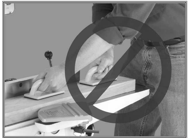
Figure 4. Never stand directly behind the workpiece!
