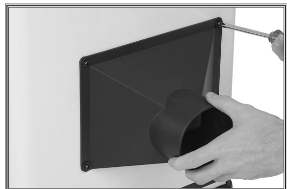
Figure 24. Attaching dust port to jointer stand.
