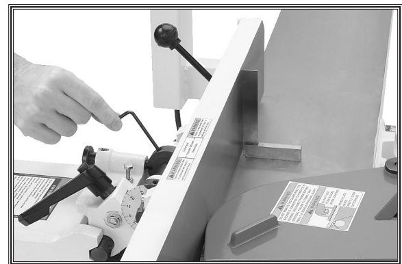
Figure 62. Adjusting fence to 90°.
