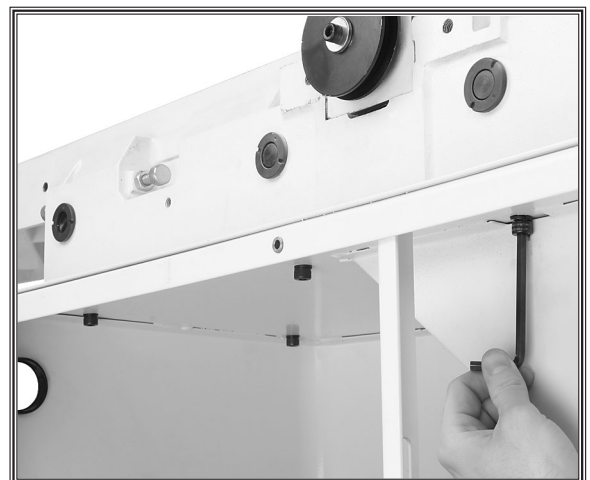
Figure 11. Securing the jointer to the stand.
