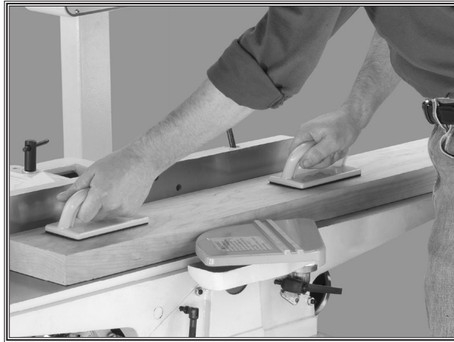
Figure 1. Correct operator and workpiece position, guard is in place, and push blocks are being used.
