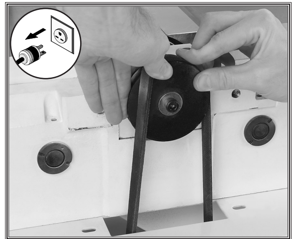
Figure 65. Rolling the V-belt onto the cutterhead pulley.
