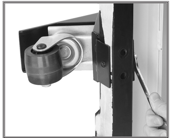
Figure 9. Bolting wheel assembly to stand.
