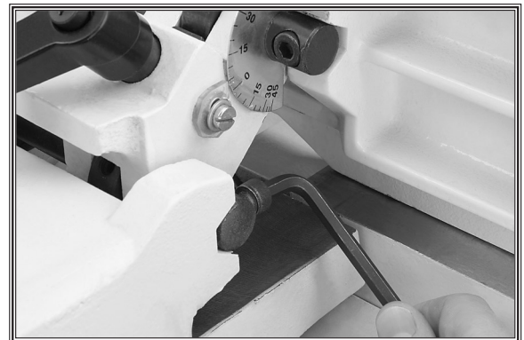
Figure 20. Attaching fence to carriage.
