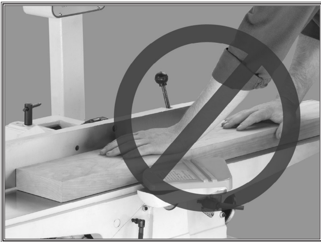
Figure 2. Never surface plane without push blocks!
