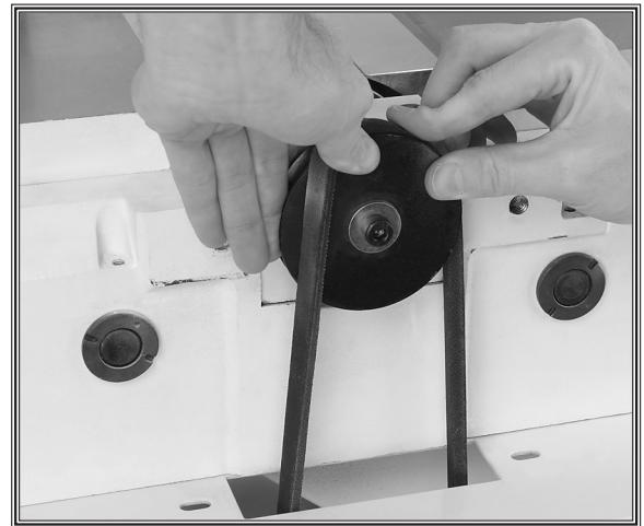
Figure 13. Rolling the V-belt onto the cutterhead pulley.
