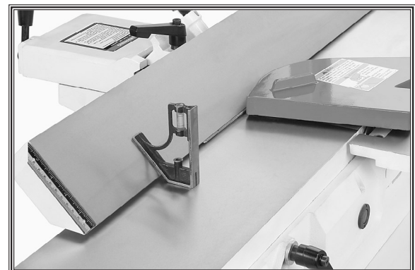
Figure 63. Adjusting fence 45° outward.
