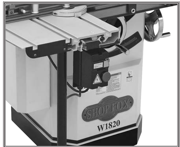
Figure 4. Example of relocating the power switch.
