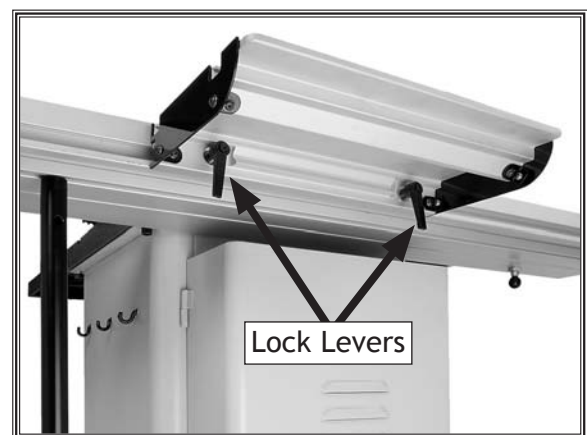
Figure 17. Locations of the extension table lock levers.
