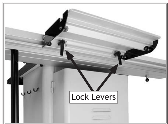
Figure 12. Locations of the extension table lock levers.
