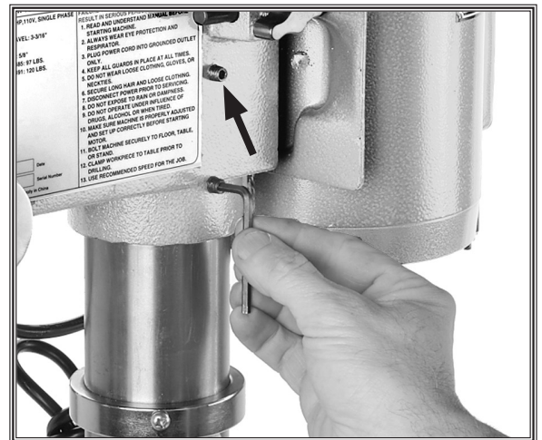
Figure 10. Securing headstock to column.
