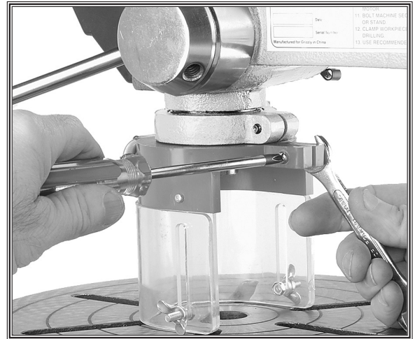
Figure 11. Installing chuck guard.
