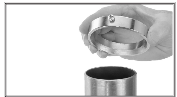
Figure 7. Correct column ring orientation.
