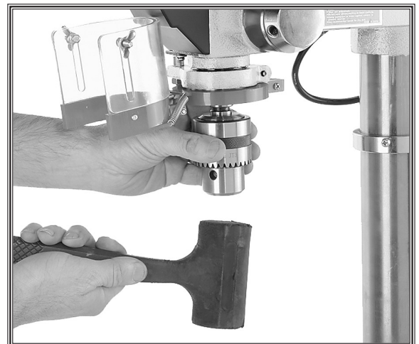
Figure 14. Seating arbor and chuck into spindle.
