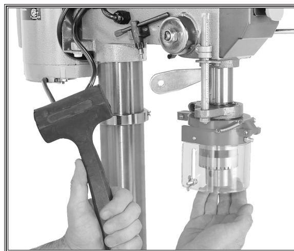
Figure 25. Using drift key to remove arbor.
