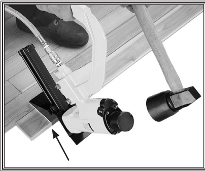
Figure 3. Positioning and operating stapler on flooring strip.
