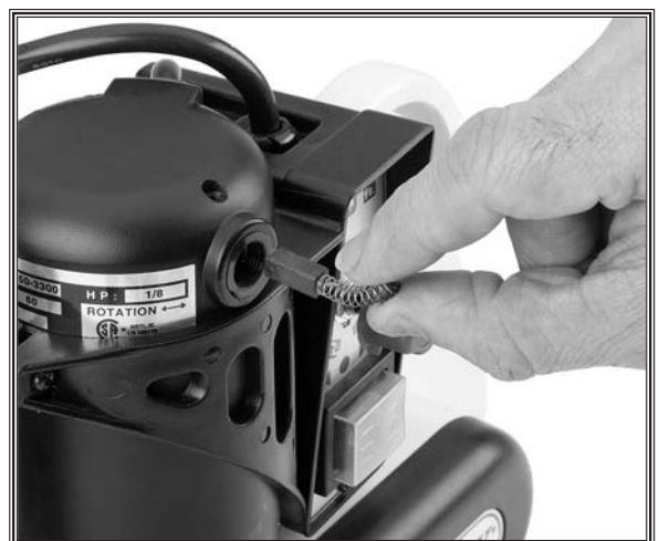
Figure 19. Brush set replacement.
