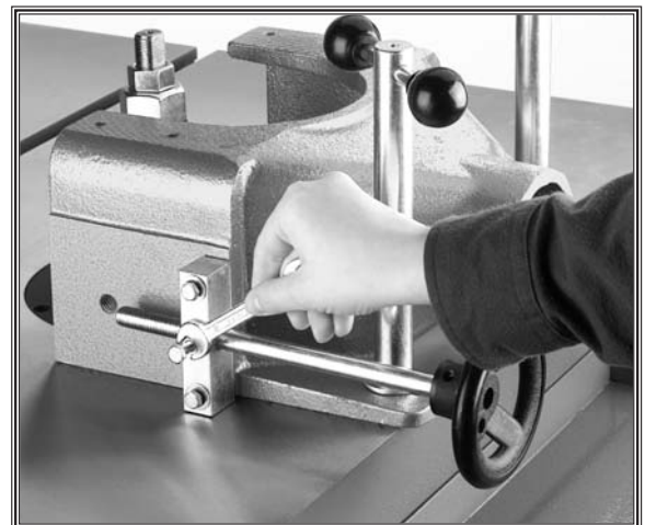
Figure 10. Installing fence adjuster.
