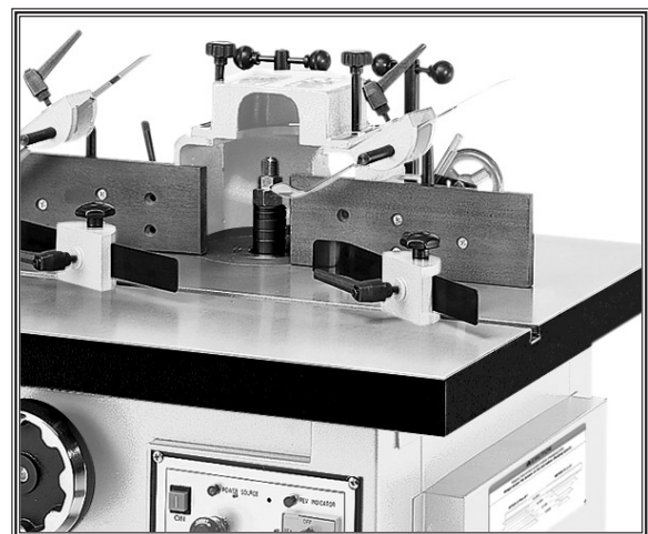
Figure 35. Hold-downs assembled and installed.
