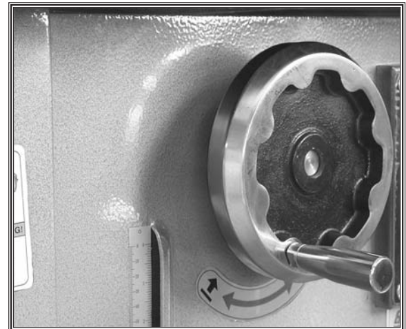
Figure 15. Handwheel handle installed.
