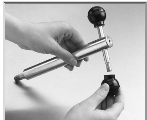
Figure 7. Installing the cross bar knobs.
