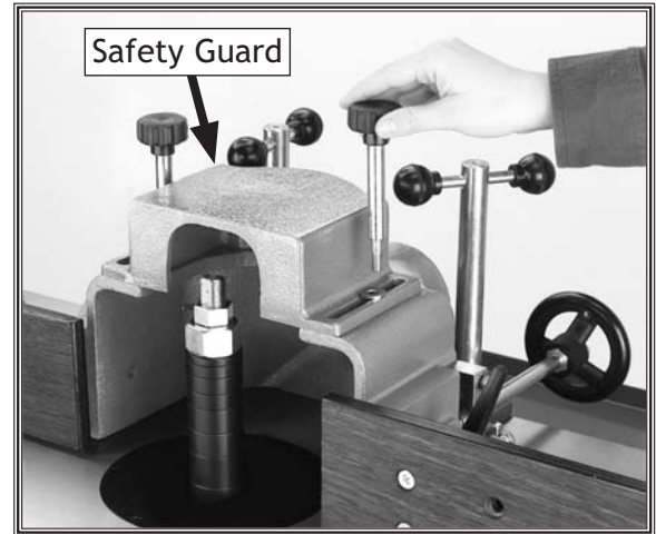
Figure 14. Installing safety guard.
