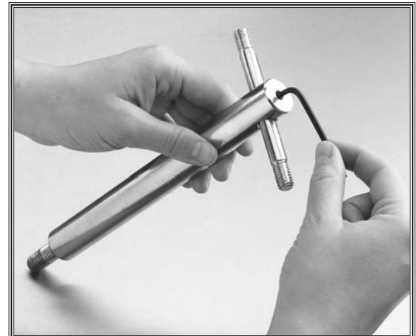
Figure 6. Securing cross bar in place.
