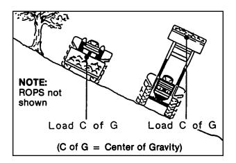
When working on side hills, **DO NOT RAISE LOADER TOO HIGH.** Keep an eye on terrain changes. Keep load low. Safety is a primary concern in the design and manufacture of our products. Unfortunately, our efforts to provide safe equipment can be wiped out by a single careless act of an operator.
